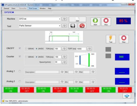
The first Digital Input will be used to received the ON/OFF of the equipment (if you are using a parts sensor, the system will allow you to configure the TOFF to filter the regular gap between parts)
