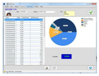
For the day selected the system shows all the changes of the ON/OFF Digital Input and duration (typical log).
